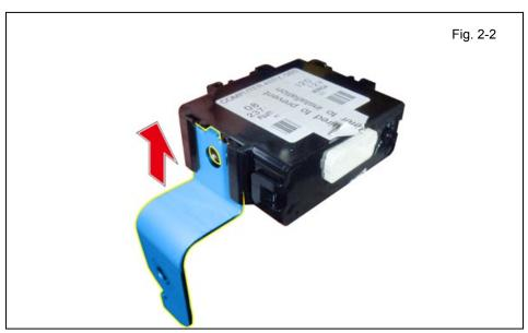
b. Attach the GBS ECU Bracket to the GBS ECU as shown.
